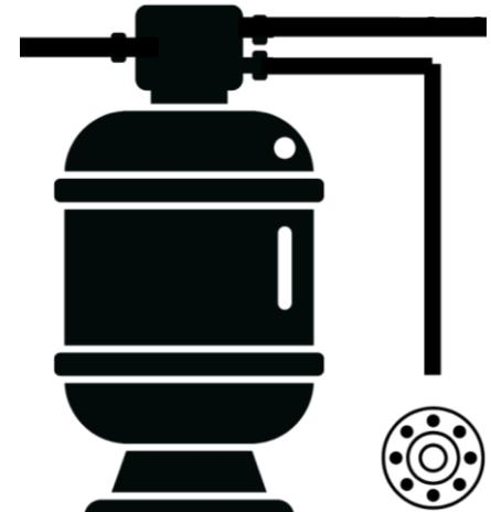
**Pressure Filters & Separation Tanks:** One or more lids that provide slow/safe release of pressure and a manual air release in addition to an automatic release with a posted sign (See Sign Table)
